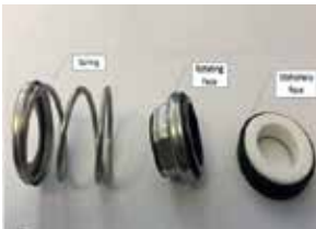
Parts of a Dynamic sealing ( Simple Mechanical seal) for a centrifugal pump
