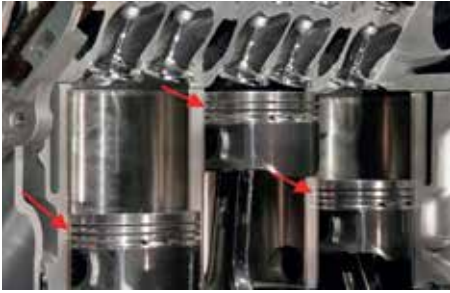
Dynamic sealing of a reciprocating piston in an internal combustion engine
